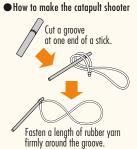
The catapult shooter allows you to fly your glider much higher than launching by hand. Use thumb and index finger to grasp below the wings, or the rearmost part of the fuselage, and launch.
