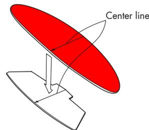
When sticking the right and left wings together, make sure that the center line is not off center.
