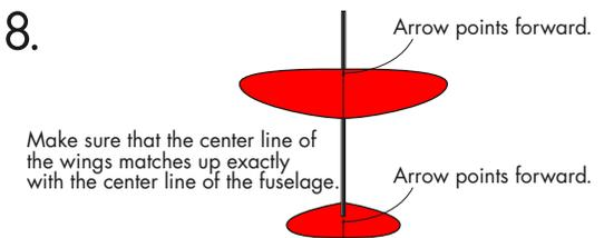
Make sure that the center line of the wings matches up exactly with the center line of the fuselage.
