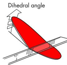
To give the wings an angle, bend along a straight ruler. (Refer to the assembly instructions for details on what degree of angle to use.)
