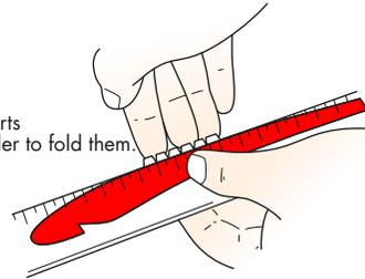
If any of the cut out parts are bent, this will seriously affect the glider's performance. Therefore, be sure to keep all parts perfectly flat till you join them up. For the wings, stabilizer and other parts, use a ruler to give you a proper straight edge to make your folds.
